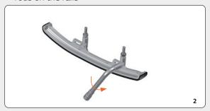
2. Loosen the adjustable sliding fixation
