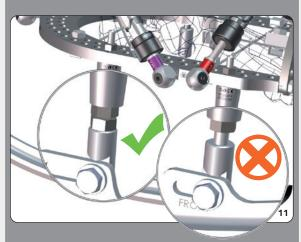
11. To adjust the distance between Foot Plate and RockerRail insert nuts and/or extended nuts between the Extender and the RockerRail. Do not allow any portion of bare rod.
