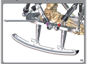
10. The larger side of the Extender must be in direct contact with the footplate
