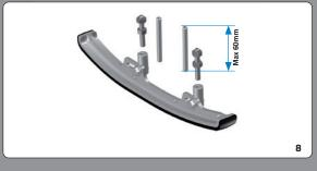
8. Exchange the rods with the threaded rods of the desired length
