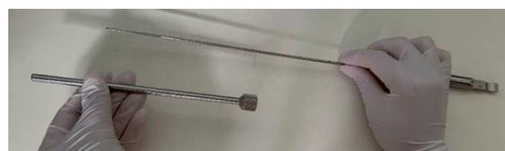
从滑块按钮左侧拆下带导向管的端帽
