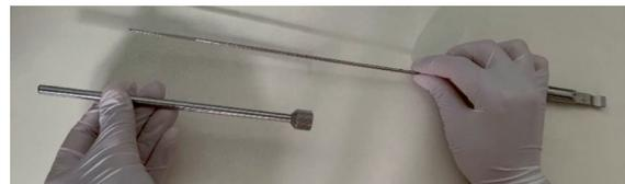
Remove cap with guide housing from button with slider on the left
