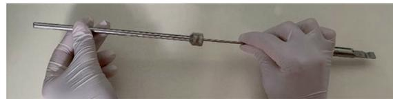
Unscrew cap with guide housing from button with slider
