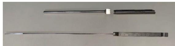
Depth gauge for sleeves disassembled
