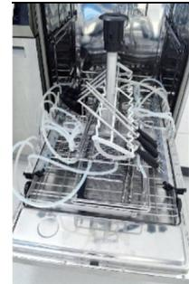
Load trays laying the instruments on the dedicated brackets, in accordance with the markings visible on the lower side of the tray lid. :
