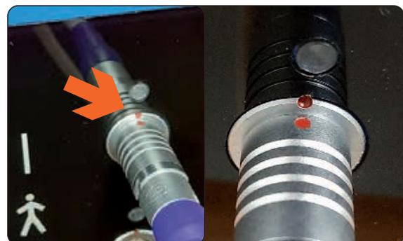
Figure 22 LINING UP THE CABLE CONNECTOR AND THE RECEPTACLE
