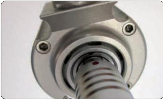
Figure 19 PLUGGING THE HANDSET CABLE INTO THE HANDSET
