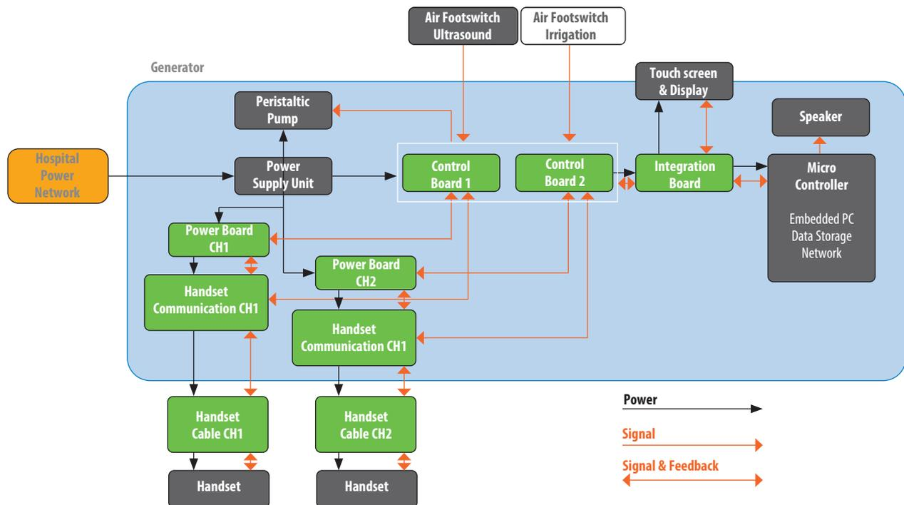
Figure 10 OSCAR PRO™ SYSTEM DIAGRAM
