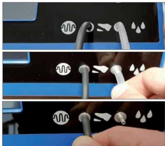
*Figure 64 DISCONNECTION OF IRRIGATION TUBE FROM GENERATOR*
