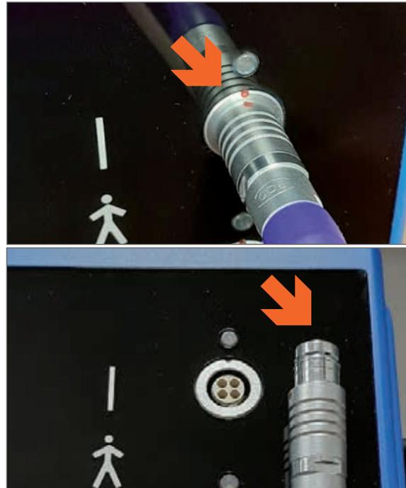
Figure 58 HANDSET CABLE DISCONNECTION FROM GENERATOR
