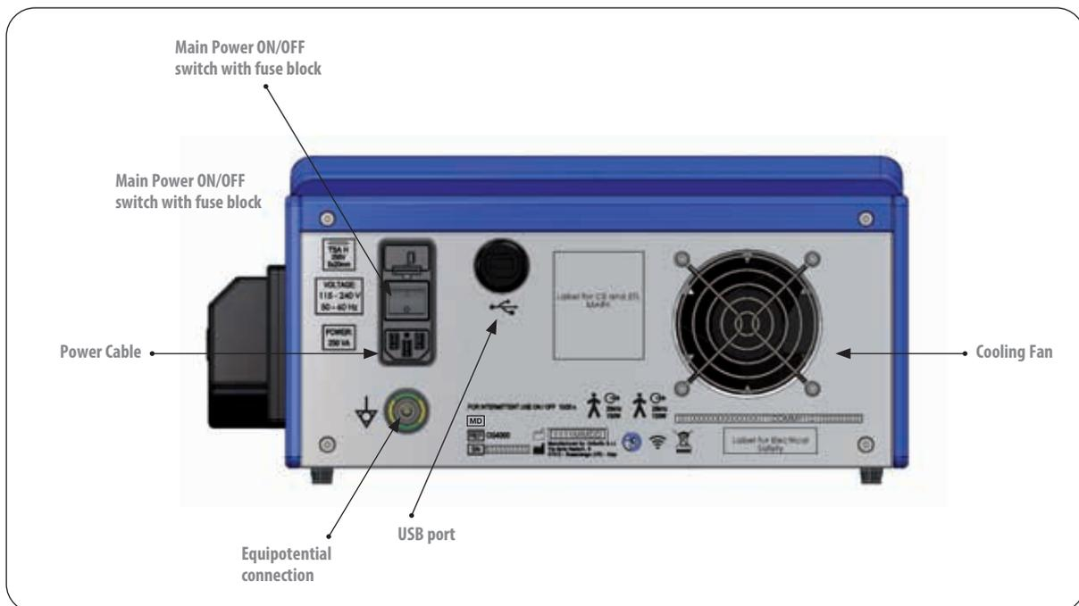
Figure 8 INTERCONNECTION DIAGRAM REAR VIEW
