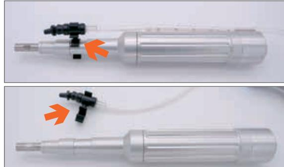
*Figure 60 WATER IRRIGATION DISCONNECTION*
