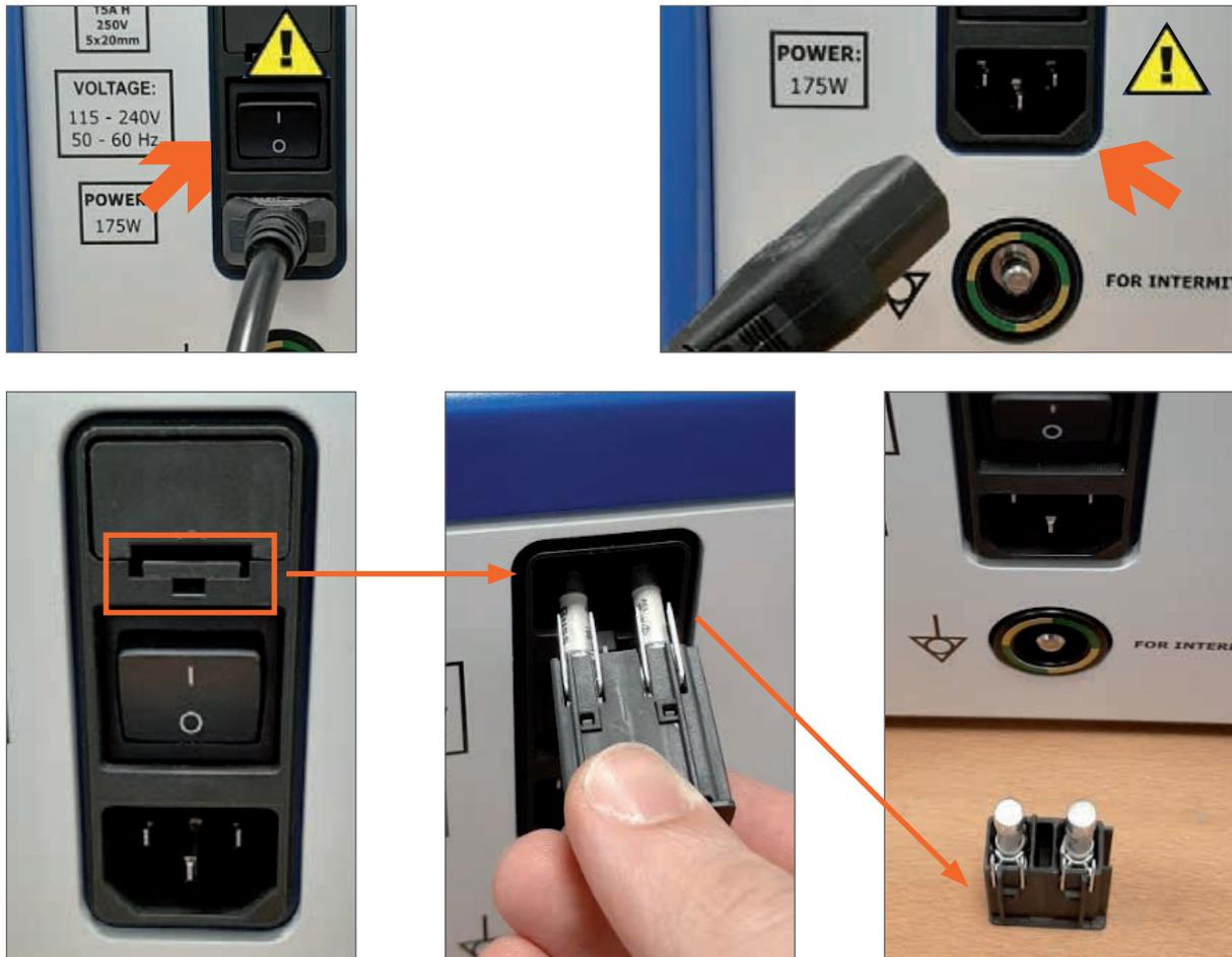
Figure 72 REPLACEMENT OF MAIN FUSES
