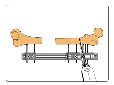
Perform osteotomy using drill bit in corresponding drill guide. Connect holes with osteotome.
