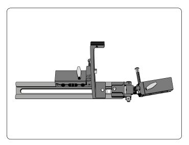
Attach angulation template; adjust to reflect varus deformity; tighten hinge locking screws.
