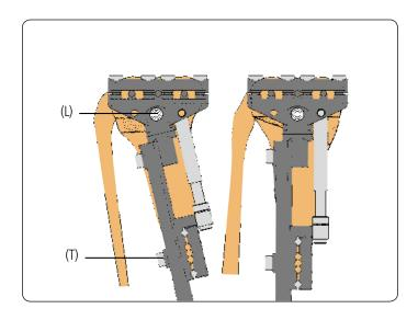
Change position of removable locking pin, and with clamp axis locking nut (L) loosened and straight clamp locking screw (T) tightened, distract to correct angular deformity. When correction complete, tighten clamp axis locking nut.
