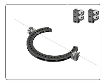
First wire may be inserted free-hand. Use a X-Wire without olive and attach it to ring using a three-hole wire clamp slider unit at each end.
