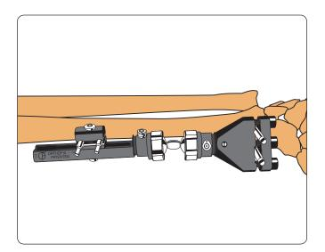
Mount the fixator with the sliding module proximally and the Extraarticular Radiolucent Wrist Clamp distally with the screw in the Lister's Tubercle housed in the fixed screw seat.
