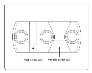
The Extra-articular Radiolucent Wrist Clamp allows for convergent placement of the second distal screw. Convergent placement may be used if the radial epiphysis is very small, but the surgeon should be aware that this type of screw placement may lead to impingement of the soft tissues and reduced bone purchase. This procedure is therefore recommended only for surgeons with substantial experience in wrist surgery.
