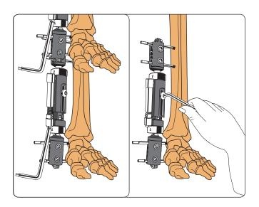
Attach the compression-distraction unit and exert compression, until good contact is felt between the joint surfaces. Avoid excessive compression in order to limit stress on the screws. Confirm contact between the two surfaces by X-ray. Finally, tighten the central body locking nut.
