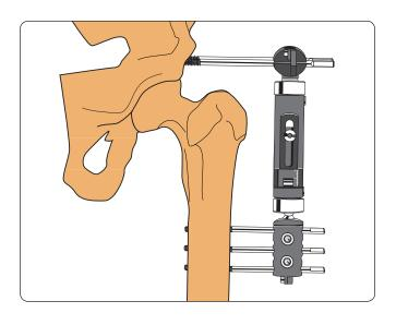
With the fixator body open by 2 cm to allow for subsequent compression, insert the three femoral screws. Prior to insertion of these screws, place the limb in the envisaged fusion position (15° of hip flexion, 5°-10° of abduction and about 10° of external rotation). Use screw seats 1, 3 and 5 in the clamp for maximal stability.
