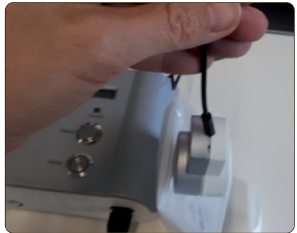
Fig. 73 Inserting the transmitter in the sterile endoscopic camera drape
