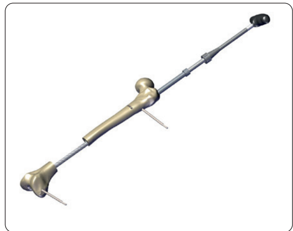
Fig. 23 Reaming of distal segment and step reamer
