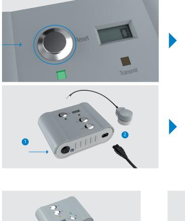
By pressing the reset button, the counter will return to 0 (zero).
