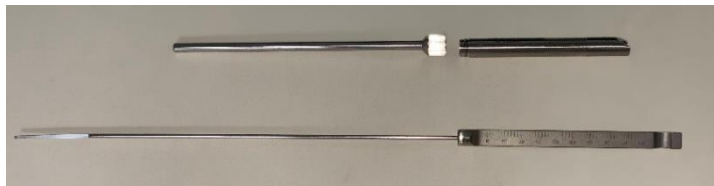
Depth gauge for sleeves disassembled
