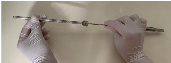
Unscrew cap with guide housing from button with slider
